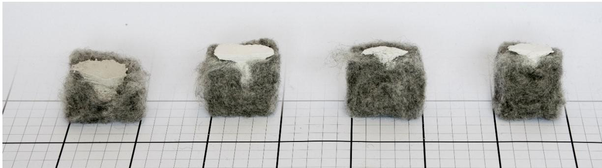
Figure 3: Sections of specimens of felted fiber. From left to right 0.032g/cm<sup>3</sup>, 0.064g/cm<sup>3</sup>, 0.096g/cm<sup>3</sup> and 0.128g/cm<sup>3</sup>. All of them infused with the same amount of plaster
